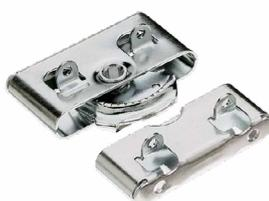
**Concealed Shallow Tab Butt-Joint Latch** Similar to the Roto Lock fastener above, however the latch and receptacle are secured with the tabs on the housing instead of the entire assembly mounted into the panel. Especially useful for quickly fitting flats and rostra. The latch and receptacle each require a 88 x 17 mm mortise in the panel 88 x 17 x 19 mm deep. These are exact sizes so some clearance may be needed. This tab mounted assemblies should be mounted with M5 screws [see page 238].
