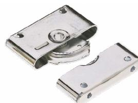
**Concealed Mortise Butt-Joint Latch** Known as a Roto Lock, these latches progressively draw panels together by means of an 8 mm Allen key [not provided] giving adjustability for theatrical tolerances or gasket shrinkage.
