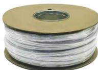
**Bell Wire** We stock this cable mainly for use with the pyrotechnic detonators. It is a twin core 0.75 mm<sup>2</sup> flexible copper wire [42 x 0.15] with a "figure 8" 0.85 mm thick PVC sheath. The cables can be easily separated.
