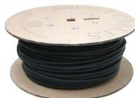
**Black Rubber Cable** This tough, black rubber-sheathed [TRS] 1.5 mm<sup>2</sup> cable is ideal for making up your own extension leads. Three core. Conformity: BS 6500 and BS 7919. Minimum bending radius: 6 x diameter.
