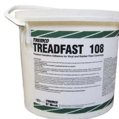
**Treadfast 108** A pressure sensitive adhesive ideal for vinyl dance floor or car carpet. It is solvent-free, non-flammable and has low toxicity. Treadfast 108 gives a strong permanent bond. Use a 1.5 mm x 5 mm notched trowel to apply and immediately roll with a short-haired paint roller dampened with the adhesive. Allow to dry [goes clear] then position and roll with 68 kg roller. Covers 6 - 8 m<sup>2</sup> per L.
