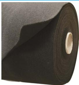
**Black Car Carpet** A useful economical black carpet ideally suited for quietening down wing spaces, off-stage rostra and get-off treads. The carpet is needlepoint rib 100% polypropylene with a latex backing. The pile weight is 400 gm<sup>2</sup> and the total weight is 450 gm<sup>2</sup>. The carpet has been tested to BS 4790:1987 [Hot Metal Nut Method].
