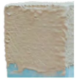
Hard foam coated with HATO®Safe and a layer of Quadraxial Fabric for reinforcement.
