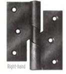
Rising Butt Hinges Designed to raise a door as it opens, the rising butt ensures that your doors do not catch on the carpet or on uneven flooring. Please ensure correct handing when ordering. The top of page 232 has all the information. These hinges tend to self-close the door as the weight of the door bears down on the bevel. They won't
