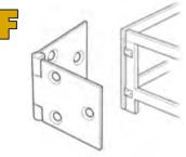
Rostrum Hinge A 2" backflap which has one flap countersunk on the opposite side to the other. These are for hinging end gates on foldinggate rostra where the hinges have to be mounted in reverse to the usual manner. A very subtle touch! It is so nice that some people are still making these lovely constructions. Steel, self-coloured.
