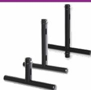
**Modular 'Tee' Frames** Available as a short version [220 - 250 mm], and a tall version [470 - 500 mm] which also has the option of a through connector style to allow the connection of another module below. All 450 mm wide and provided with tapered pins at connection points.
