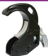
**Twenty Clamp** The Twenty Clamp is an aluminium pressure die cast clamp designed to suspend luminaires up to 20 kg. This clamp can be secured to tubes with a diameter of 48 - 51 mm with just two turns of the Doughty Knob. Luminaires are secured via a captive M10 or M12 Bolt [M10 supplied]. Damage to tubes and trussing is eliminated by using an extruded trigger. This product is fully TUV Approved. Design Registered.
