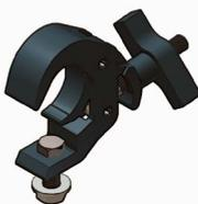
**Triple E Hook Clamp** Designed primarily for the rapid attaching of Triple E tab tracks to truss or flying bars from 38 - 52 mm but equally suitable for attaching lanterns. Width: 30 mm. Weight: 578 g
