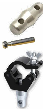
**Connector** Required to link each of the modular components. Tapered pins are supplied with each module, but spares also available. The half connector has an M12 internal thread for attachment via a bolt to a clamp or eye of your choice. We can supply a wide range of these connectors, see our website for further details. The Doughty Clamp version listed here has a SWL of 100 kg and weighs just 780 g.
