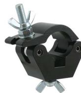
**"Hook" Clamp** Very popular high tensile aluminium clamps widely used for attaching scenery as well as lanterns to bars and trussing. Suited to large and heavy luminaires. Width: 50 mm. Weight : 710 g.
