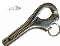
**Pelican Hooks** A convenient means of quickly releasing tensioned wire ropes. They can be very useful for clearing gauze guide wires during scene changes. To use the threaded version we will need to roll-swage an M8 right-hand thread to the end of your wire which will need to be stainless steel. Please phone and ask for the Rigging Manager. Safety factor 4:1.
