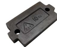
**Counterweights** Our 10kg\* Counterweight has two large holes with rounded entries to allow ropes or karabiners to pass through for hauling to the fly floor. Supplied self-colour. We also hire Counterweights [page 358]. Delivery charged at cost. \*Weights can vary plus or minus 5%. Prices are for each weight. We also supply Temporary Counterweight Cradles [page 200]. Size: 325 x 153 x 42 mm [Lug width: 60 mm].
