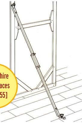
**Stage Braces** Extendable braces like these are used to support lightweight scenery. They are secured to the flats with a screw eye which locates with the hooks on the brace. The foot is designed to marry with our stage weight but it is also drilled for use with either Stage Screws or Stage Bolts into Boss Plates [page 132]. Made from tulipwood with bright zinc-plated fittings. We also include a small brace, useful for ground rows. Special sizes can be made to order.
