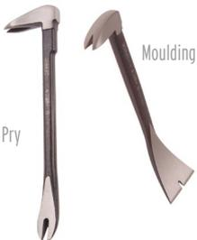
**Stanley Pry Bars** Two very effective designs. The heads can be struck with a hammer to grip under embedded nails. They will pull out headless and rusted nails or screws. The wide end of the moulding pry bar allows the user to cleanly pry off delicate mouldings. Pry bar: 300 mm long. Moulding pry bar: 200 mm long.
