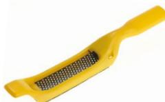
**Stanley Surform 21-102** This flat file with a 140 mm blade has a GRP handle with a thumb screw to adjust the blade. Ideal for smoothing glass fibre, body filler, nylon and wood. Can be used in environments that would ruin a decent plane.
