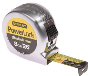
**Stanley Powerlock Tape Measures** Comes with a chromium-plated plastic case, removable belt clip, a Tru-Zero end hook and a power return with sliding lock. The yellow blade with black markings has a Mylar coating which increases blade life by up to ten times. The 8 m tape also has transparent blade armour on the first 150 mm for maximum durability and reduced breakages. Marked with both metric and imperial markings. Replacement blades available to order. For Tape Pouches see page 328.
