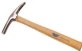
**Magnetic Tack Hammer** This solid forged head tack hammer features a magnetic fork face to aid placement of the nail when hammering. Head coated with a lacquer for improved rust protection.
