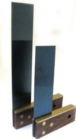
**Carpenter's Try Squares** Made to BS 3322, these try squares come in "Plantation grown" rosewood with a 1/8" [3 mm] brass facing strip. The hardened, tempered and blued steel blade is fixed to the wood stock by brass rivets.
