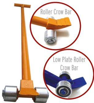
**Roller Crowbars** For serious shunting of heavy scenic units. Ideal for rescuing heavy trucks after a castor has collapsed or got jammed in a track. Essential equipment for fitting-up heavy steel scenery and trucks to align bolt holes or for general servicing of castors. We stock two types. Full details can be found on page 359.
