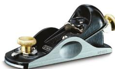
**Stanley 9 $\frac{1}{2}$  Block Plane** The classic block plane has been in use for over 100 years. The cutter is fitted at 21° and is adjustable for depth and alignment. The mouth can be set for fine or coarse work. The perfect tool for removing the arris from timber to prevent splinters. Its handy size makes it a good choice for a touring tool kit.
