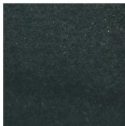
**Super Wool Serge 500-525 g/m<sup>2</sup>** DFR. Black. Wool serge provides the best material for masking. This heavyweight fabric is durably fire retardant and has less sheen than velour. Perfect for covering masking legs and borders or for making tabs. Serge is not normally glued to flats but
