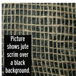
**Jute Scrim 85 g/m<sup>2</sup>** Not FR. Natural colour. An open weave jute scrim normally used to reinforce plaster waste moulds but could be used to reinforce and add texture to large scale polystyrene carvings. Recommended glues include FlintsBond and Sheppy M155.
