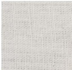
**Super Scenic Flax 360 g/m<sup>2</sup>** NDFR. Bleached white. This is the standard material for covering open framed timber flats prior to painting. Recommended glues include warm size and Clam 2 or use Sheppy M155 if gluing large areas to plywood. Sold per metre.
