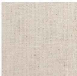
**Calico 195 g/m<sup>2</sup>** NDFR. Natural colour. A good economical lightweight material suitable for covering plywood clad flats. Calico, being rather lightweight, will not disguise poor joins between ply sheets which may need filling [see page 57 for suitable fillers]. If the surface is very poor, cotton canvas
