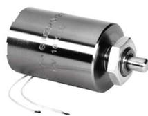
**Small Shot Bolt** This device is ideal for light-duty safety catches on safety cages and lift access gates. They spring to lock and energise to release. It can also be used to drop light loads. It has a 10 mm stroke on its 8 mm diameter
